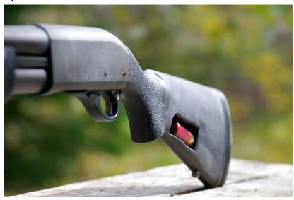
SpeedFeed stocks (now discontinued) were available from Remington on certain Police and Marine Magnum XCS models. It used a unique spare shell carrier built in to the stock where one could carry two extra shells on each side, held in by coil springs.
